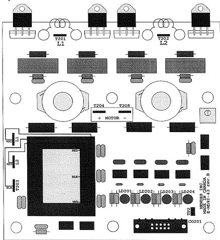
The electrical power to each DC motor is supplied through the E-MD92-43 using four terminal connectors (T201, T202, T203 & T204). Each DC motor is protected by an overload located on the front of the electronic power box with the electric circuit being completed through the terminal circuit board (E-MD92-21).
