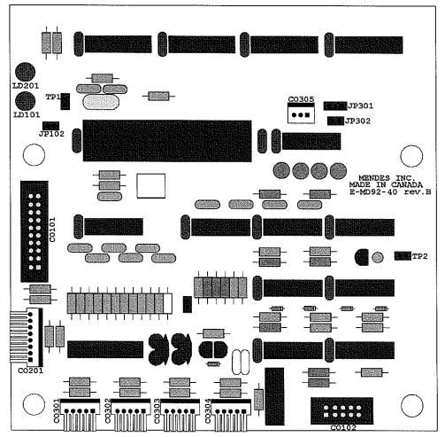
The E-MD92-40 communicates with the main circuit board (E-MD92-92) through an MTA connected to CO101. It is through the main circuit board that each motor is turned ON and OFF.
